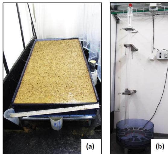
**Figure 1.** The rainfall simulation flume (a), and the settling tube apparatus (b). The settling tube apparatus consists of four components: the settling tube, through which the soil sample settles; the injection device, by which the soil sample is introduced into the tube; the turntable, within which the fractionated subsamples are collected; and the control panel, which allows an operator to control the rotational speed and rest intervals of the turntable (operations see Hu et al., 2013b).
