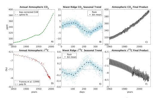
**Figure 2.** Niwot Ridge synthetic data product for atmospheric CO<sub>2</sub> concentration ( $c_a$ ) (**a**, **b**, **c**) and  $\delta^{13}$ C of CO<sub>2</sub>( $\delta_{atm}$ ) (**d**, **e**, **f**). The final time series (**c**, **f**) were used as a boundary condition for CLM, and created by combining the annual trends reported by Francey et al. (1999) adjusted for Niwot Ridge (**a**, **d**) with the mean seasonal cycles measured at Niwot Ridge (**b**, **e**).
