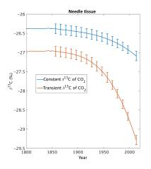
**Figure 6.** Simulation of  $\delta^{13}$ C of needle tissue using the limited nitrogen (default) CLM run. In the constant  $\delta^{13}$  C of CO<sub>2</sub> ( $\delta_{\text{atm}}$ ) simulation the model boundary condition was  $-6\%_o$ , whereas the transient  $\delta_{\text{atm}}$  simulation varied over time (Fig. 2).
